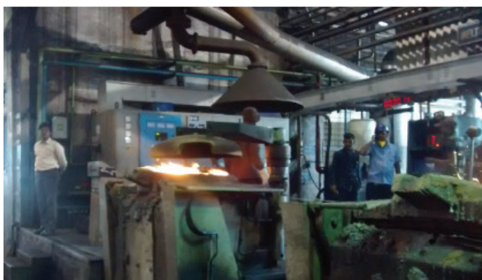
Figure 12: Induction Furnace Lid Mechanism
